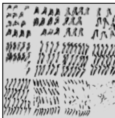
Figure 2—Classification of dry hobbled chips and their form groups.
